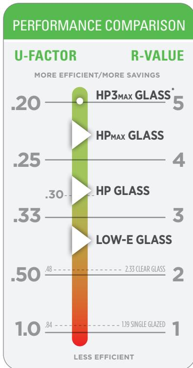
The lower the U-Factor, the greater the insulation value. R-Value is the inverse (R=1/U) of the U-Factor. Total Unit Factors determined per NFRC-100 (National Fenestration Rating Council). Chart shows relationship between performance and Ply Gem Windows & Doors glass package options, not including energy package upgrade.
